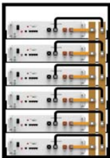
Figure 5-1 Schematic diagram of battery connection
