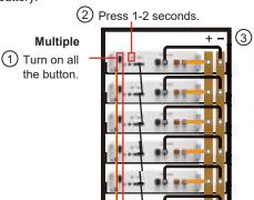
(3) Wait a few seconds and the batteries will automatical turn on one by one, until all the running lights flash,indicating that the batteries are working properly.
