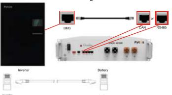
Note: Please connect the master battery and the inverter. Multiple
