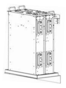
Insert the main body into the base components, and fix both sides with 4 screws.
