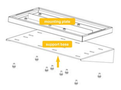
2 Fix the base components on the wall with 10 expansion bolts.
